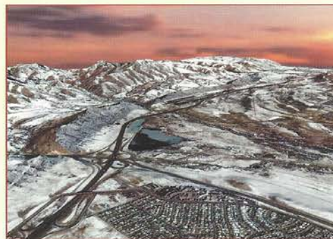
IKONOS Drape: Space Imaging, Inc. captured this winter scene south west of Denver using IKONOS satellite. The image was orthorectified to 3.5 meters horizontal accuracy using an Intermap DEM, and electronically draped over the DEM to create this perspective.
