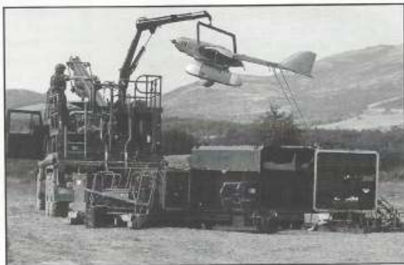
Phoenix is transported in all-weather, air tight containers. It is assembled by the soldiers and loaded by crane onto the "rail" where it is launched. Photographer: QMSI K Andrews RLC
