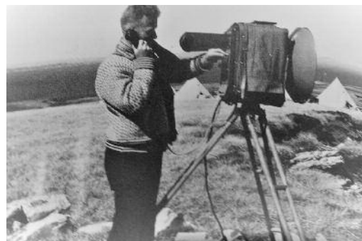
Operating the MRA1 Tellurometer at Wreck Gate trig point, North Arm 9 Dec 1958.
