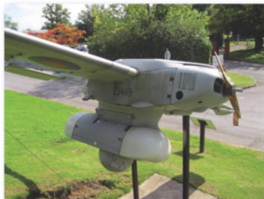
The Phoenix UAV, with an infra-red camera mounted in a stabilised pod, was launched from a truck-mounted hydraulic ramp. It was deployed to Kosovo, Macedonia and Iraq.
