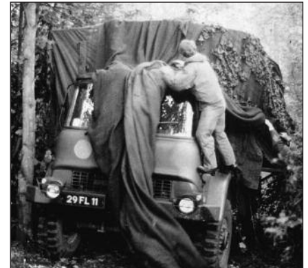
Crew member in NBC kit 'camming up' a 19 Squadron MAPSP on an exercise.
