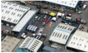
Figure 2 – Snapshot of a 3D model of a site of interest for the investigation, created on-site from 30 overlapping oblique high resolution images. The model was used for pre-mission briefings and to confirm dimensions of buildings and vehicles.
