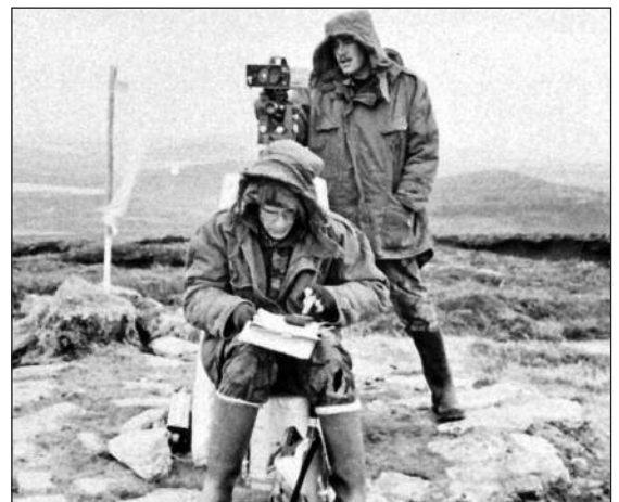
Sapper Whitehead (driver) observing with Corporal Boulton (field surveyor) booking on Benbecula – many drivers became competent assistant surveyors.
