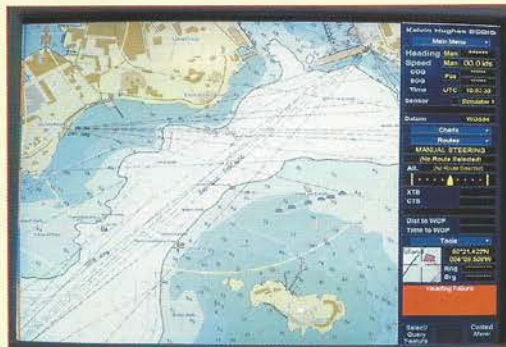
An ECDIS screen displaying an ENC (Electronic Navigational Chart).
