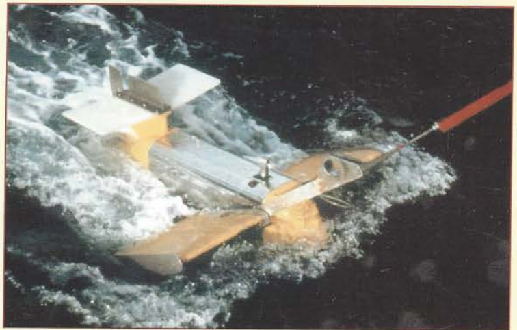
Chelsea Instruments new improved SeaSoar Mark II open ocean towed undulating data acquisition vehicle
