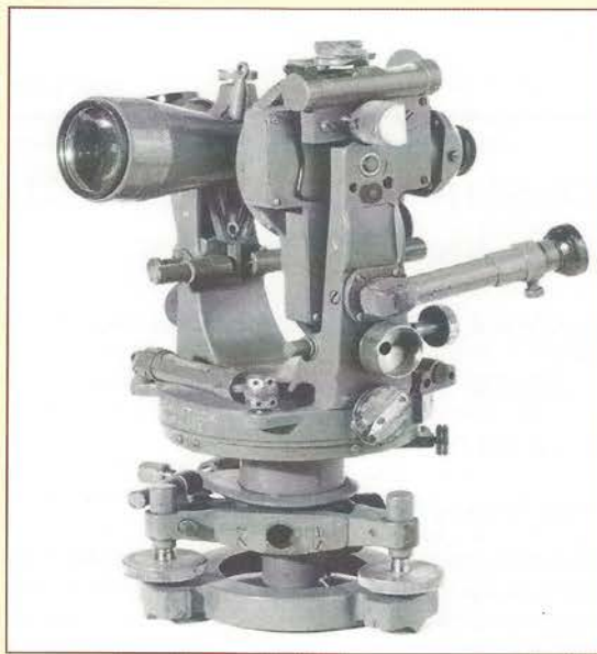
The renowned Tavistock theodolite.
