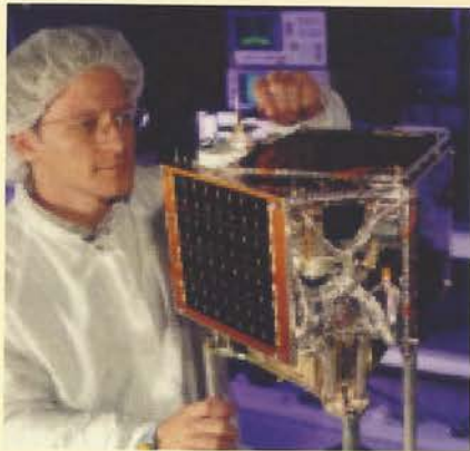
Fig 7: SNAP for 6 - 12 kg payloads with GPS orbit determination, three-axis attitude control and micro-propulsion (Image courtesy Surrey Satellite Technology Limited)
