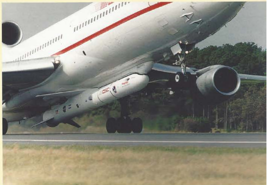
Fig 6: Orbital Sciences Pegasus launcher on take off underneath L-1011 Stargazer with OrbView-3 (Image courtesy: Orbital Sciences Corporation)
